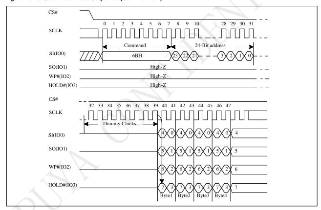
Figure 10-15 Quad Read Mode Sequence (Command 6B)
