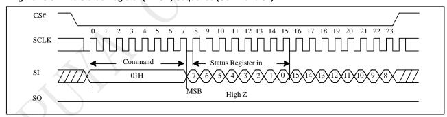
Figure 10-8 Write Status Register (WRSR) Sequence (Command 01)
