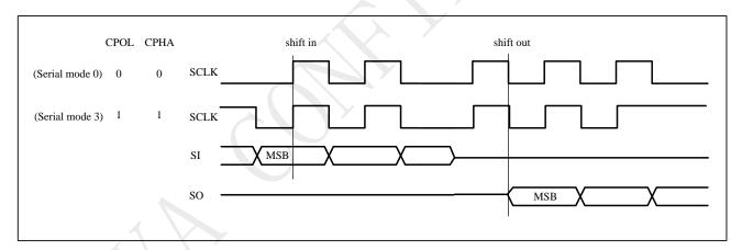
Figure 8-1 Serial Peripheral Interface Modes Supported
