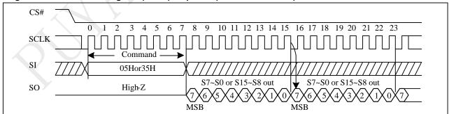
Figure 10-5 Read Status Register (RDSR) Sequence (Command 05 or 35)
