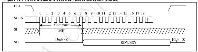
Figure 10-7 Active Status Interrupt (ASI) Sequence (Command 25)
