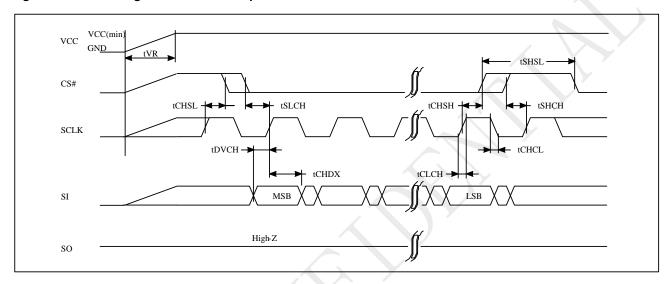
Figure 5-9 Power-up Timing
