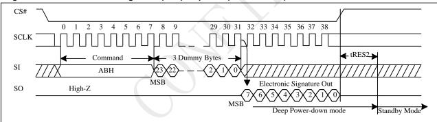
Figure 10-31 Read Electronic Signature (RES) Sequence (Command AB)
