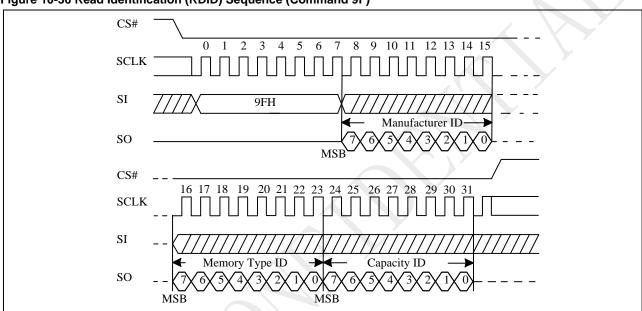
Figure 10-36 Read Identification (RDID) Sequence (Command 9F)
